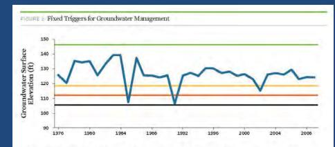
In this example, the threshold for chronic lowering of groundwater levels is the lowest groundwater elevation recorded (black line). Fixed triggers have been set at the land surface elevation (green-light trigger), one standard deviation (yellow-light trigger), and two standard deviations (red-light trigger) below the average groundwater elevation. The blue line represents the data, which are recorded depth-to-groundwater measurements over time. Union of Concerned Scientists 2015
