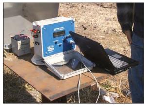
C. Data logger, encoder, and satellite-transmission equipment
